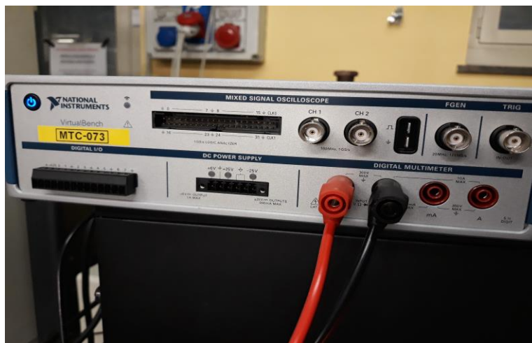
Figure 5.3 VirtualBench used to measure the resistance
