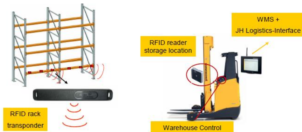
Figure 40: RFID tags on shelf and on forklift
