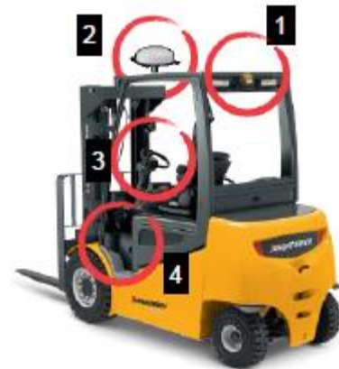
Figure 44: RTLS hardware on forklift
