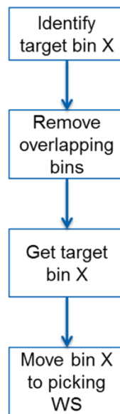
Figure 17: Picking process of Autostore AGV
