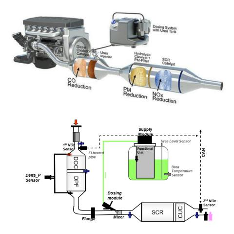
Fig. 31- Exhaust Gas ATS layout
