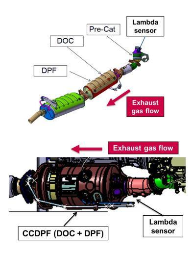
Fig. 32- ATS Layout – Oxygen sensor detail
