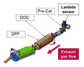
Fig. 42- Upstream Oxygen sensor
