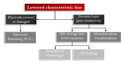
Fig. 49 - Failure tree flow chart
