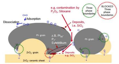
Fig. 48 - Example of Three Phase Boundary contamination
