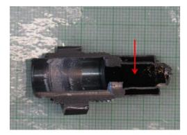
Fig. 51 - Protection tube. Presence of soot indicated.
