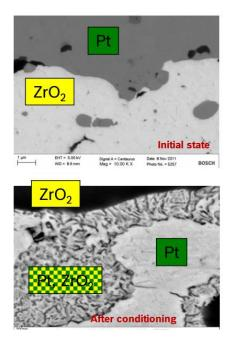
Fig. 59 - Comparison between TPB without and with conditioning process
