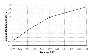
Fig. 34 - Output voltage trend respect to A/F ratio
