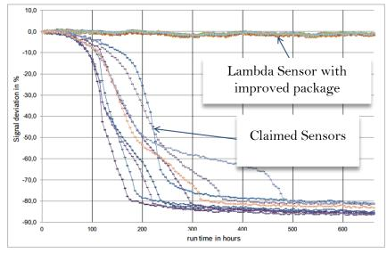
Fig. 60 – Signal deviation in component air test
