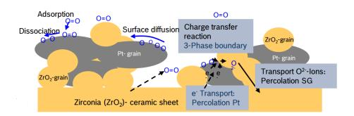
Fig. 57 – Three Phase Boundary working principle
