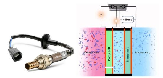
Fig. 33- Oxygen Sensor case (left) and Sensing Element working principle (right)
