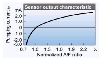
Fig. 45- Output pumping current characteristic
