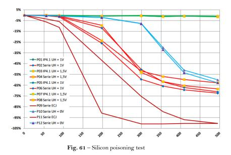
A silicon poisoning test was also performed. From the trend shown in Fig. 61 is possible to verify that no deviation due to silicon occurred.
