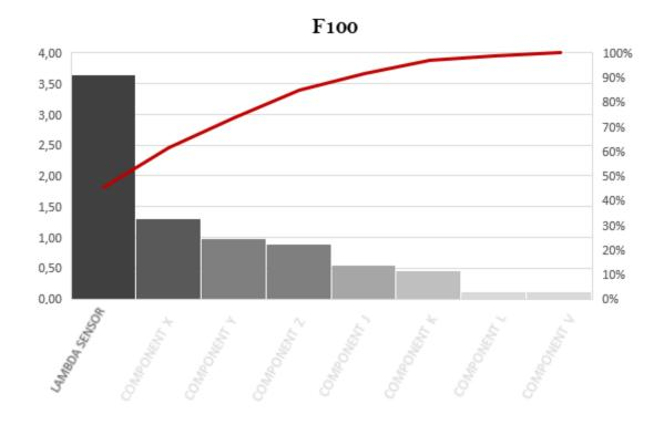
Fig. 40- Most critical failure rate of ATS components
