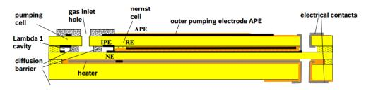
Fig. 44 – Sensing element detail
