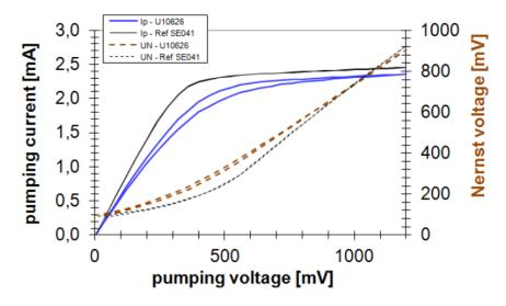
Fig. 47 – Pumping current drifting respect to pumping voltage
