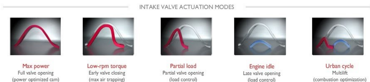
Figure 26 - Multi-air characteristics (VVA by FCA)
