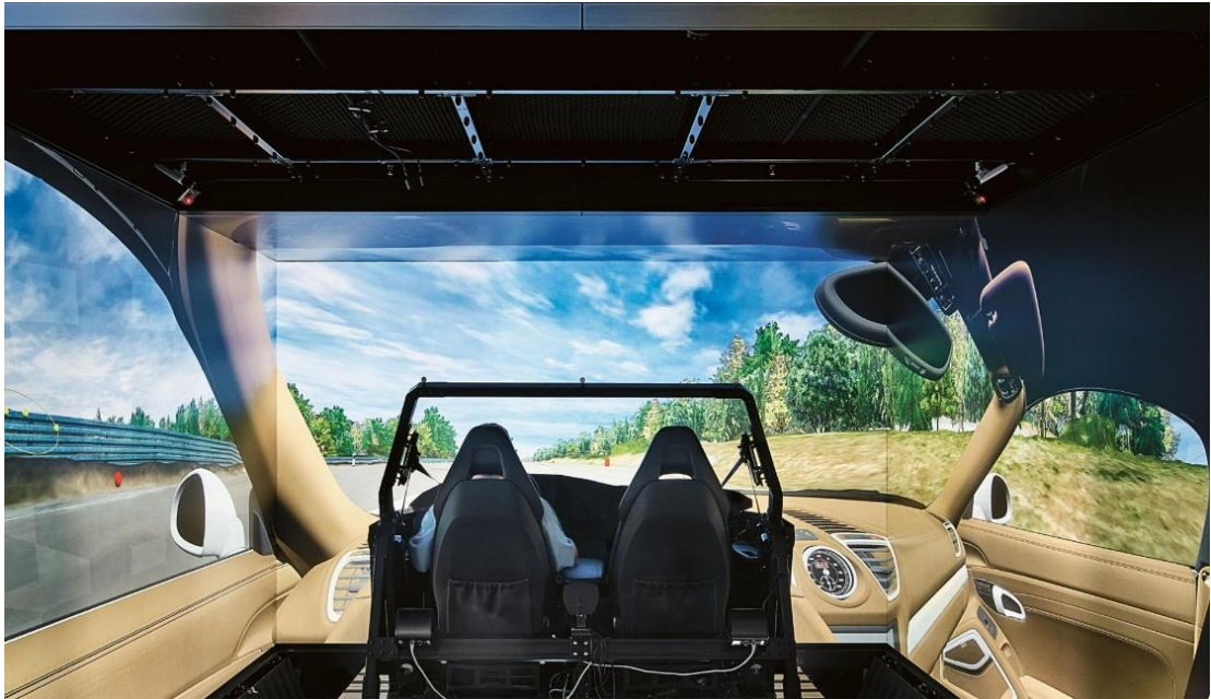
Figure 3.1: CAVE with physical seating-buck as interaction with the virtual environment (From Porsche Newsroom)
