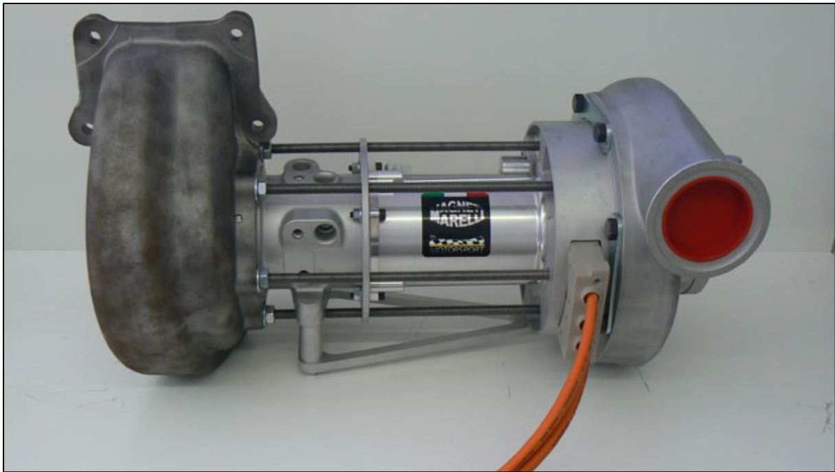
Figure 2.4 The "MGU-H" by Magneti Marelli, used in F1 world championship 2014
