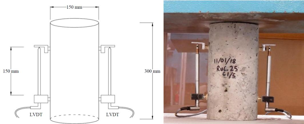
**Fig. 42** – Compressive strength test configuration
