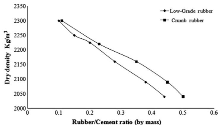
**Fig. 14** – Influence of type and quantity of rubber on density of concrete (Fattuhi and Clark, 1996).
