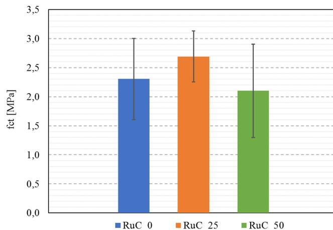
**Fig. 53** – Average tensile strength values
