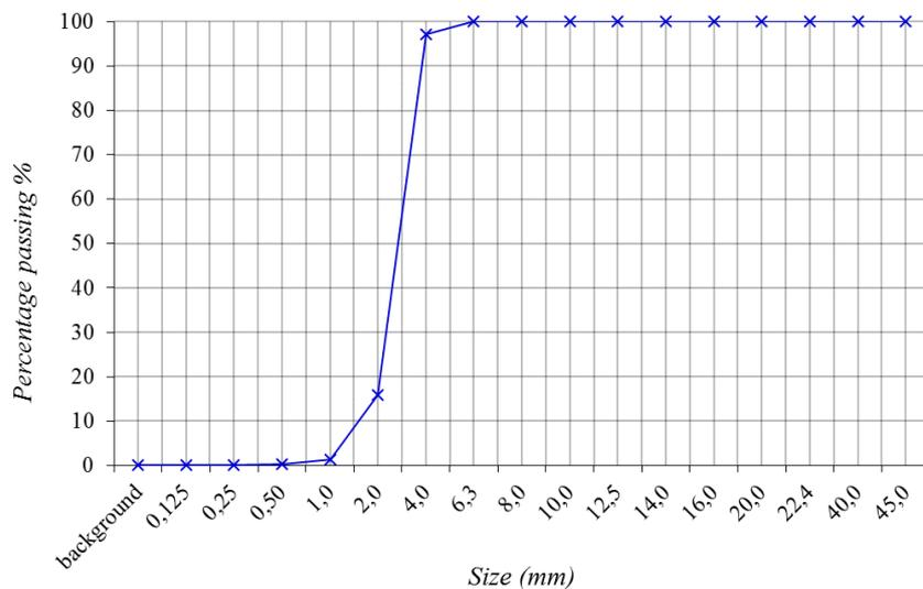
**Fig. 28** – Sieve analysis for waste rubber aggregate
