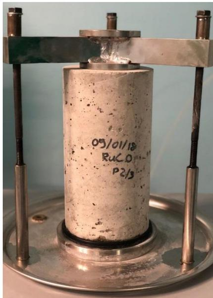
Fig. 46 – Permeability test
