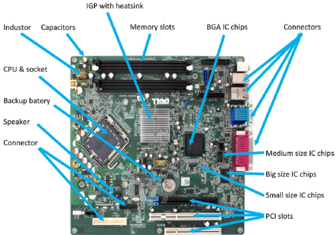
Figure 3.1. Motherboard of a scrap PC. Source: Razi [2016]
