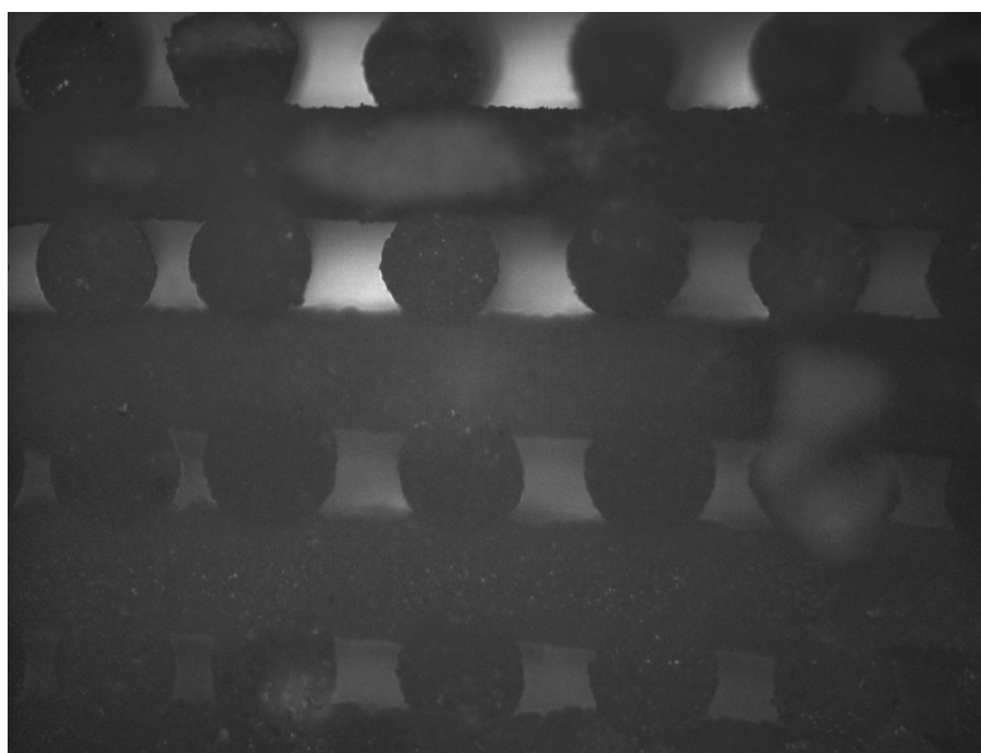
Figure 5.22 Cross-section of graded scaffold in the area of larger porosity (Optical microscope, 50X)
