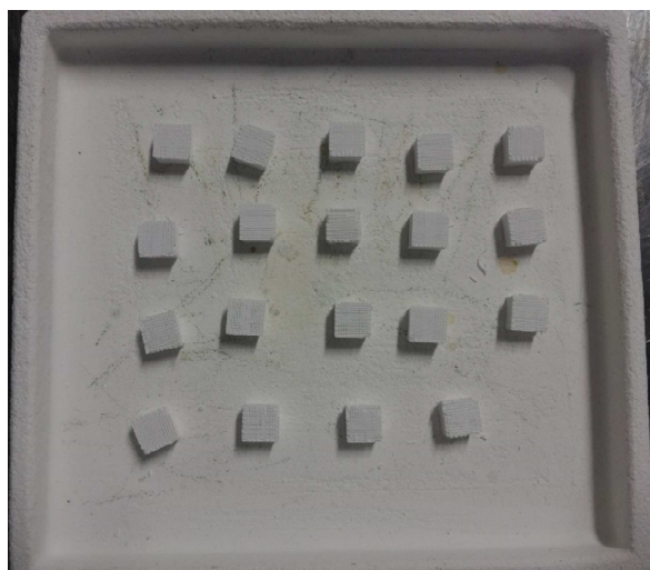
Figure 4.12 Scaffolds displaced on the alumina plate before sintering
