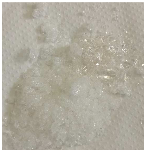
Figure 4.3 47.5B glass frit obtained by quenching molten glass in water
