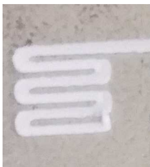
Figure 5.14 Deformed rods due to low scanning speed/high material feed
