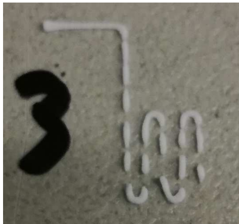
Figure 5.13 Rod brakeage during the printing of the first layer due to insufficient pressure/material feed
