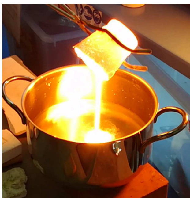
Figure 4.2 Glass casting in water to obtain a frit
