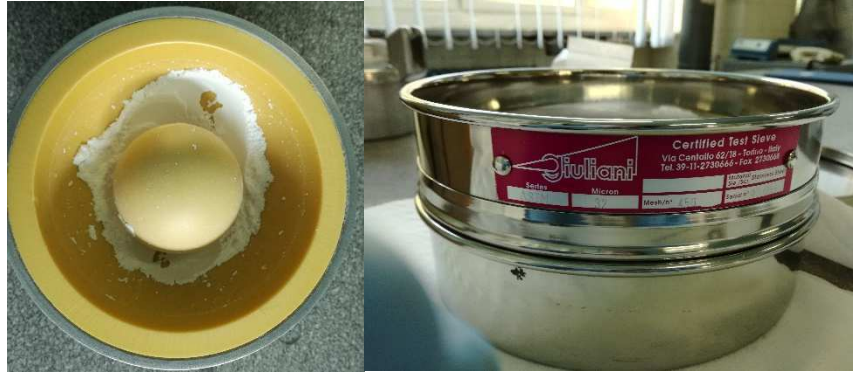
Figure 4.4 left: Ball mill with powders inside; right: the sieve used in the process
