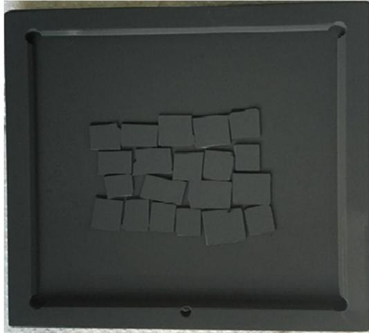
Figure 3.2: Overview of Zn thin films on Si substrates.
