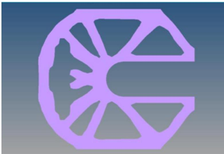
This plot provides the information about the element density. Iso Value retains all of the elements at and above a certain density threshold.
