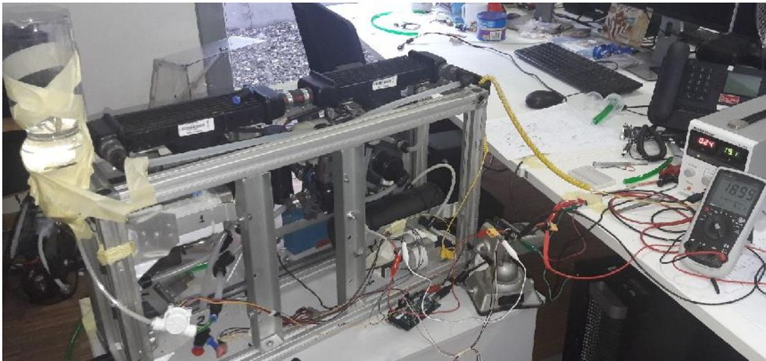
*Figure 51. Water pump test set*
