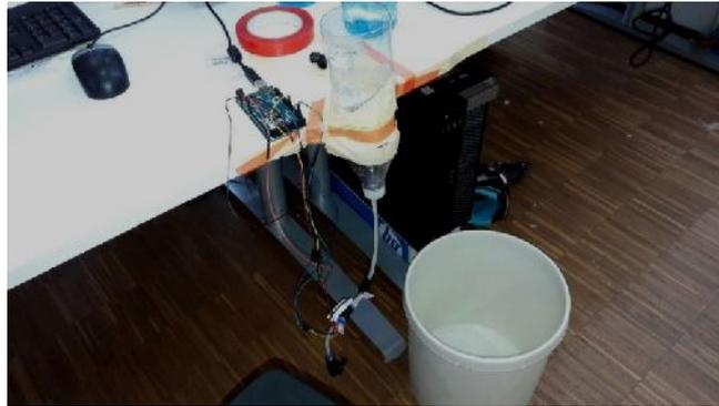
Figure 43. Water flow meter test set-up
