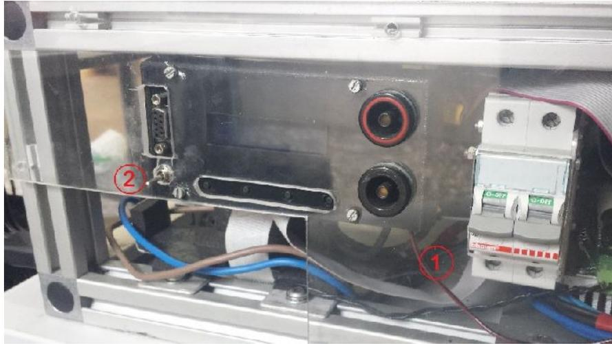
Figure 38. Master switch (1) and start operations switch (2)
