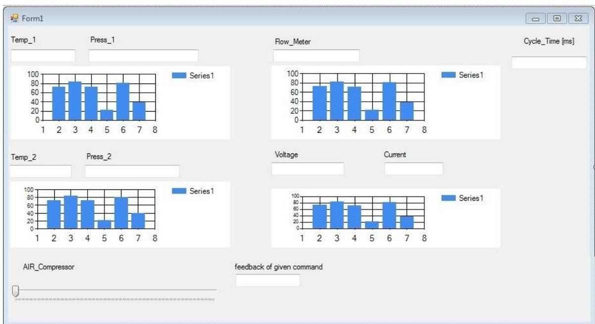
*Figure 40. Graphical interface in Vb.NET. Default interface pattern while the program is not running*
