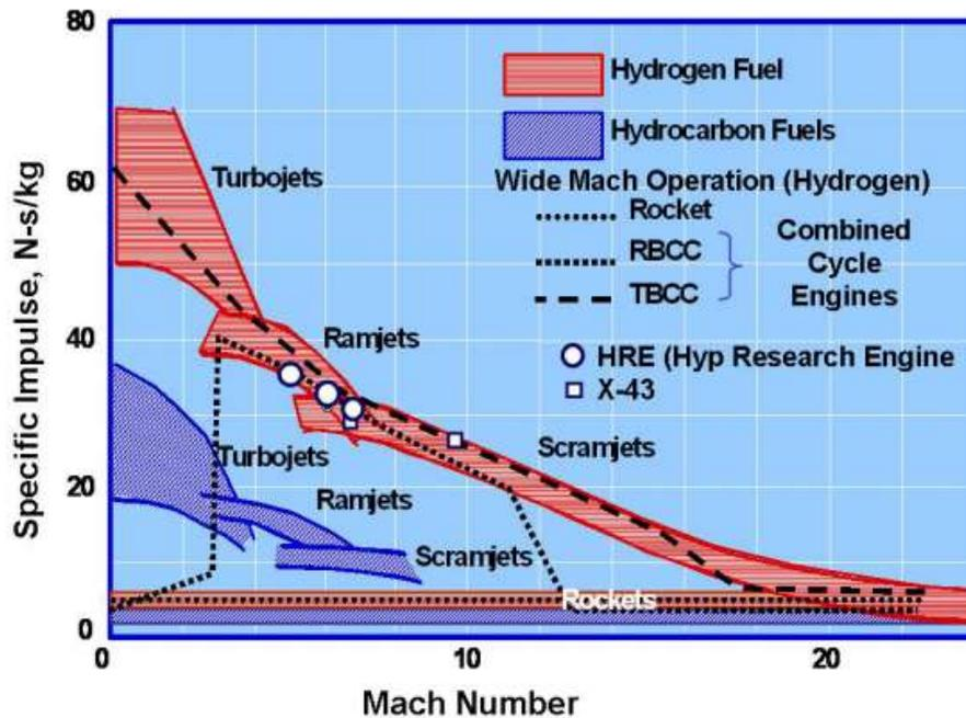
Figure 51: Hypersonic engine efficiency [40].
