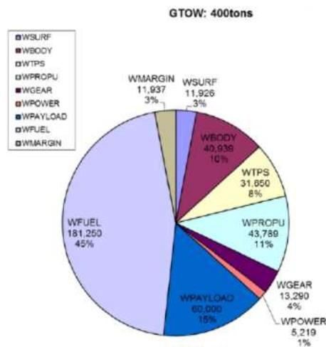
Figure 36: GTOW Mass break-down of LAPCAT MR2 [35].
