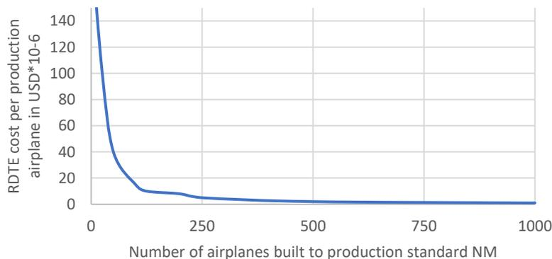
Figure 7: Effect of number of airplanes produced on the RDTE cost contribution per airplane (data from [3]).
