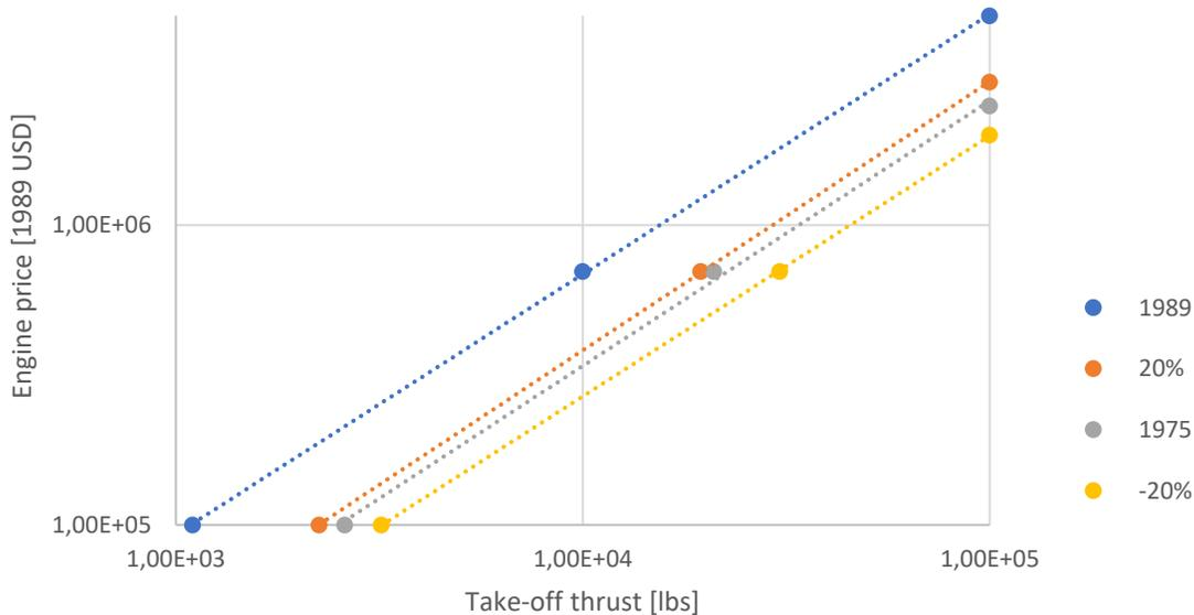
Figure 80: Relationship between engine price and the thrust at the take-off [3].
