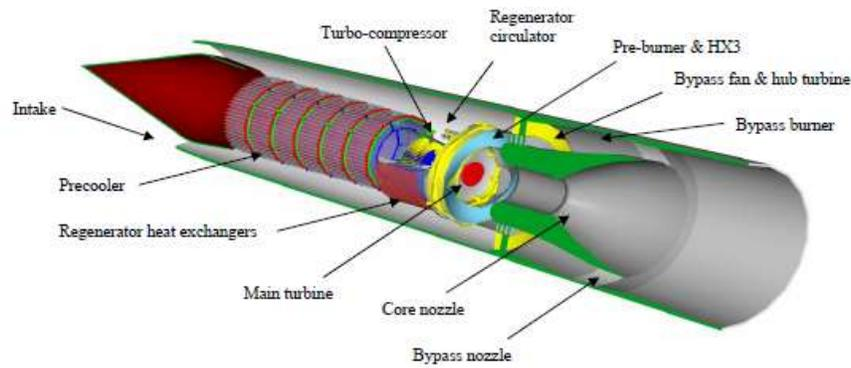
Figure 40: Section through Scimitar Installation [38].
