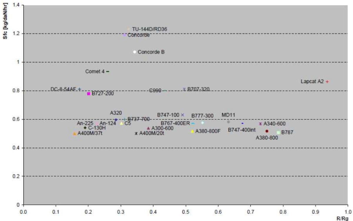
Figure 92: Indicative specific fuel consumption values for various sub- and supersonic aircraft in function [65].
