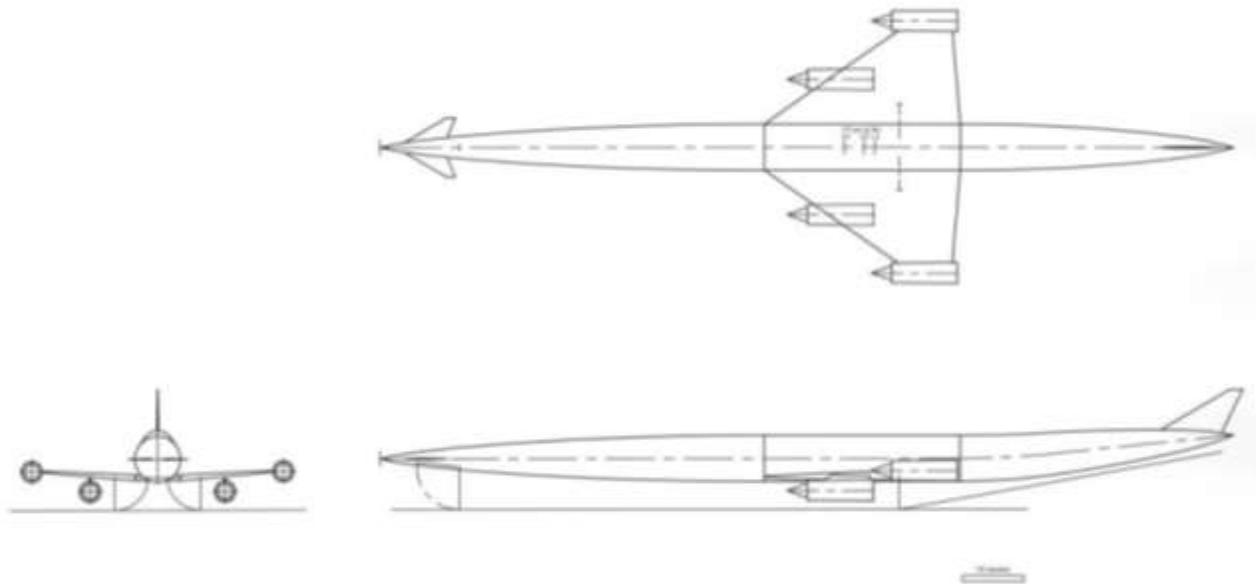
Figure 37: LAPCAT A2 configuration [36].
