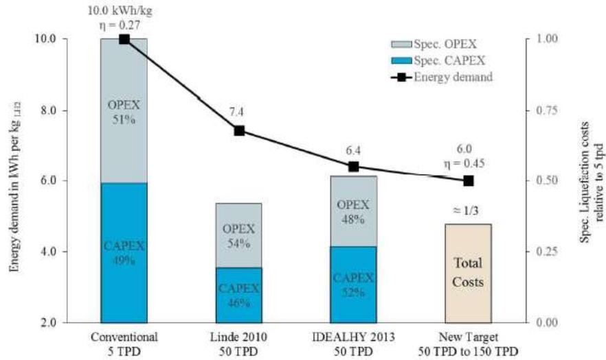
Figure 55: Liquefaction energy demand and costs of conventional and conceptual liquefiers [48].
