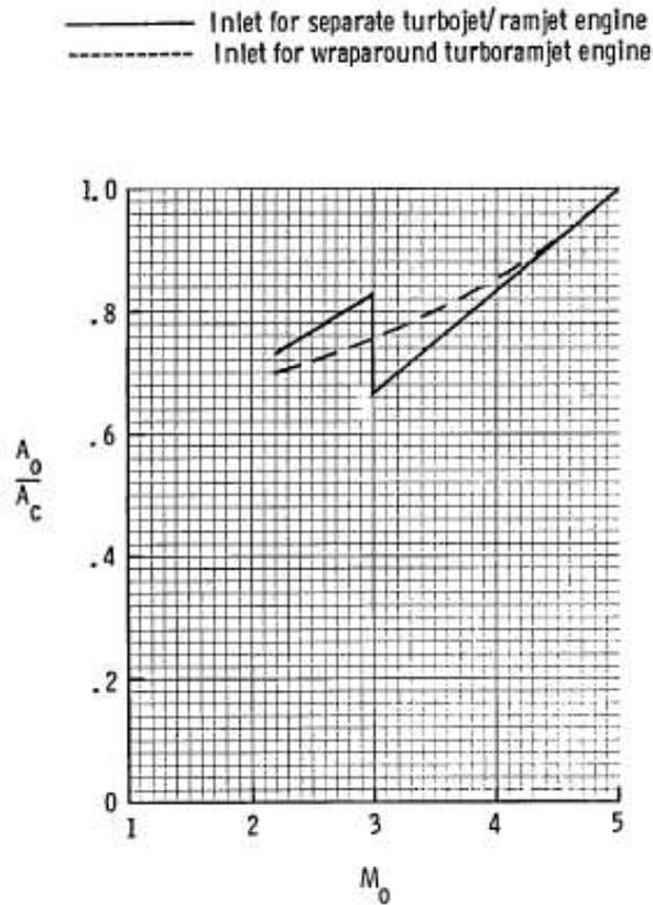
Figure 79: Inlet flow mass flow ratio for Mach between 2 and 5 [61].
