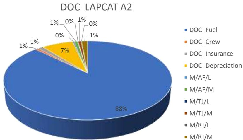
Figure 81: Direct Operating Cost for the LAPCAT A2
