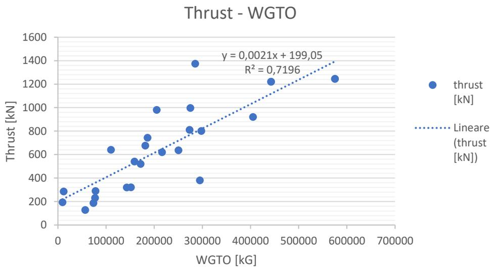
Figure 64: Relationship between the take-off weight and the thrust at the take-off.
