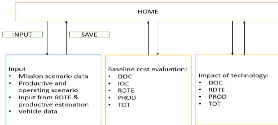
Figure 68: Chart of the final MATLAB tool for the cost evaluation of a Cruise Air Vehicle
