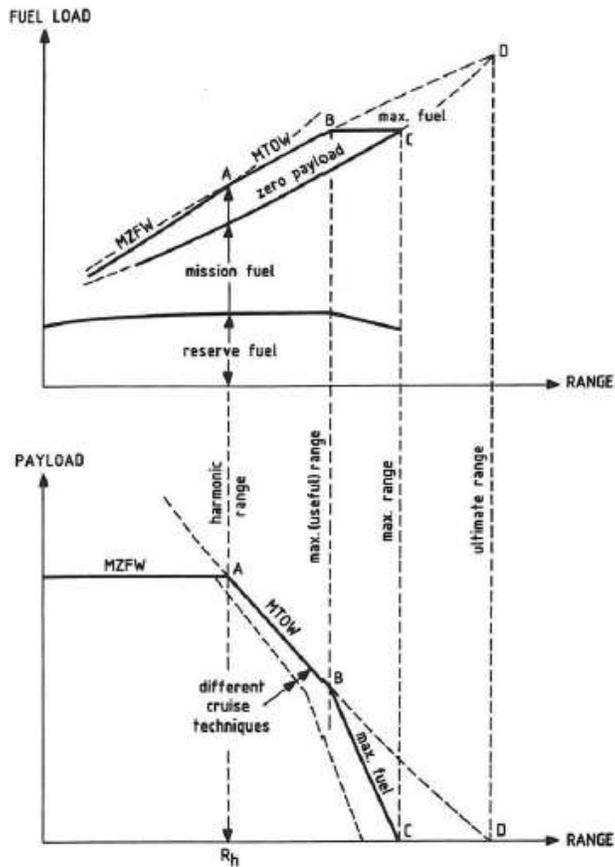
Figure 54: Payload and fuel load envelope versus range [45].
