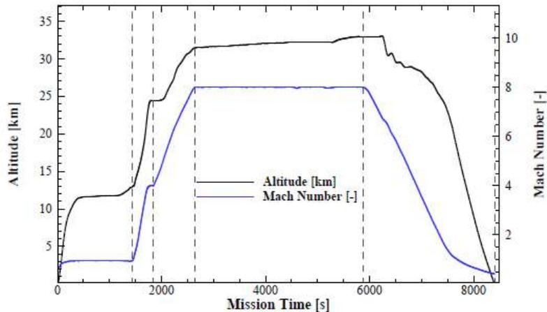
Figure 22: Mission profile of hypersonic point-to-point vehicle [24].
