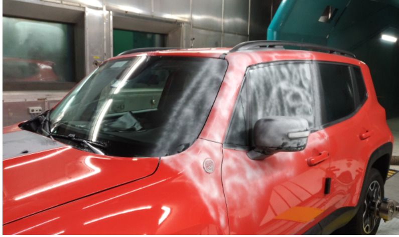
Figure 4.28: Talk is sprayed on the area of interest in order to track the path of water rivulets.
