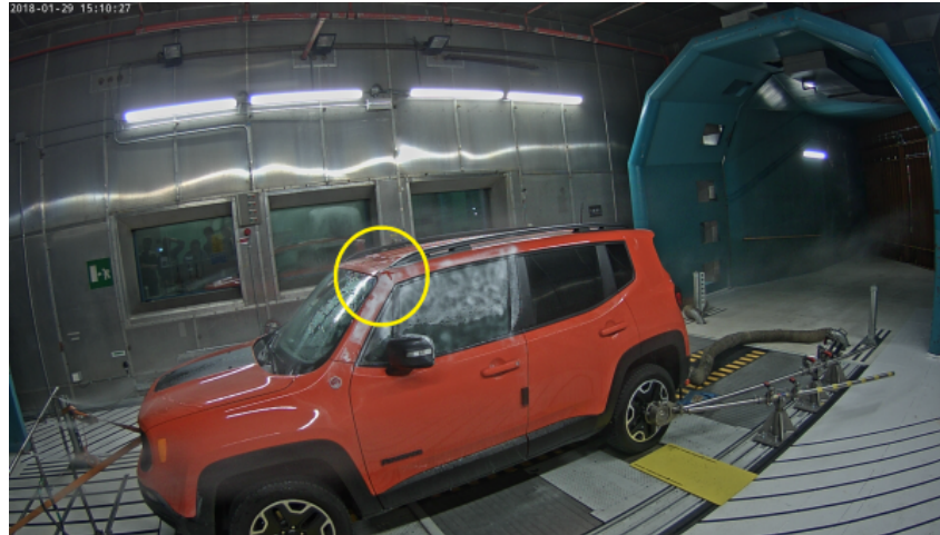
Figure 4.29: After two minutes water accumulates in the area highlighted by the circle.
