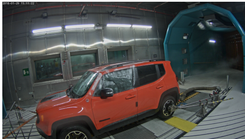
Figure 4.30: After three minutes water has overcome the A-pillar and has fallen on the side glass.
