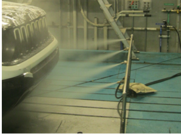
Figure 5.3: Picture of the water spraying system used in the Slipstream test. Courtesy of FCA
