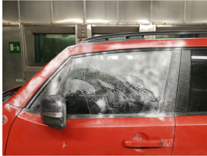
Figure 4.31: The path of water rivulets is tracked by the talcum powder. The picture is taken after the test.
