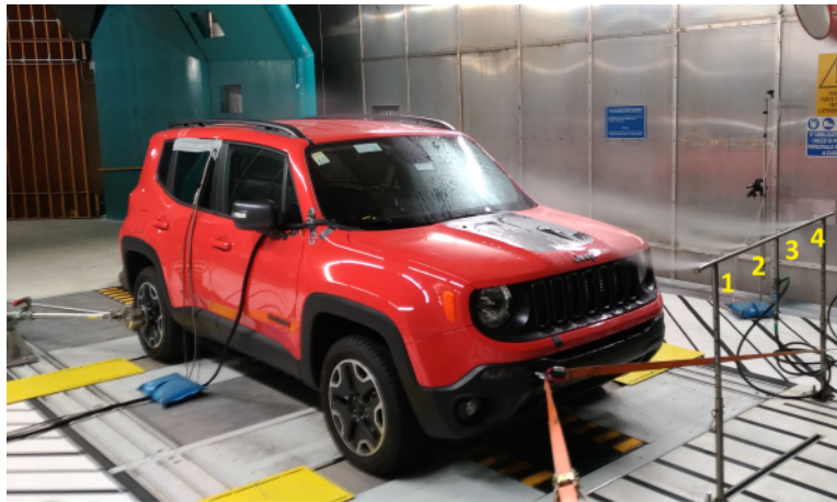
Figure 4.27: Position of the four nozzles during the water soiling experimental test. Courtesy of FCA
