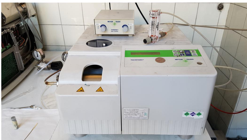
**Figura 4.18:** TGA-DTA Mettler Toledo 1600
