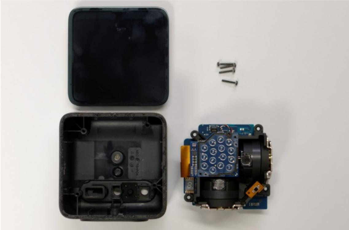
Figura 4.6: HTC Vive: in dettaglio una base station disassemblata. In alto a sinistra si notano i led infrarossi. Sul lato sinistro ed inferiore gli emettitori laser. <https://www.pcper.com/reviews/General-Tech/SteamVR-HTC-Vive-depth-Lighthouse-Tracking-System-Dissected-and-Explored/SteamV>
