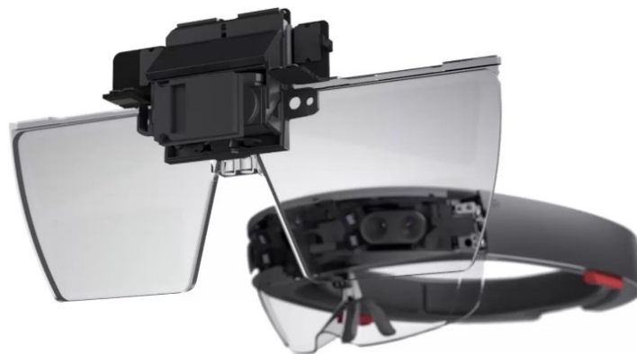
Figure 3.4. Hololens' display system, Waveguide Lens
