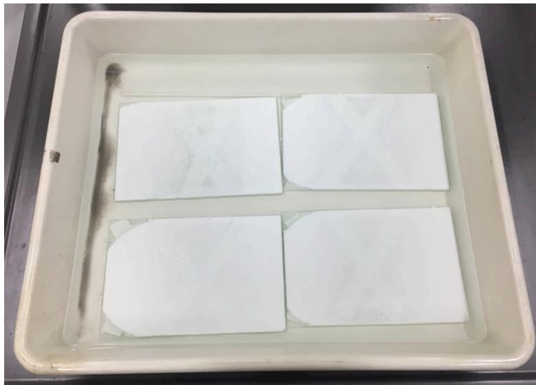
**Figure 3.13:** Membranes immersed in the coagulation bath.
