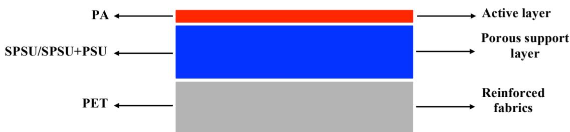
**Figure 3.1:** Schematic representation of a TFC membrane structure.
