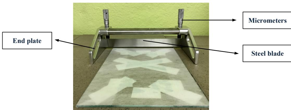
**Figure 3.9:** Gardco Microm II film casting knife.
