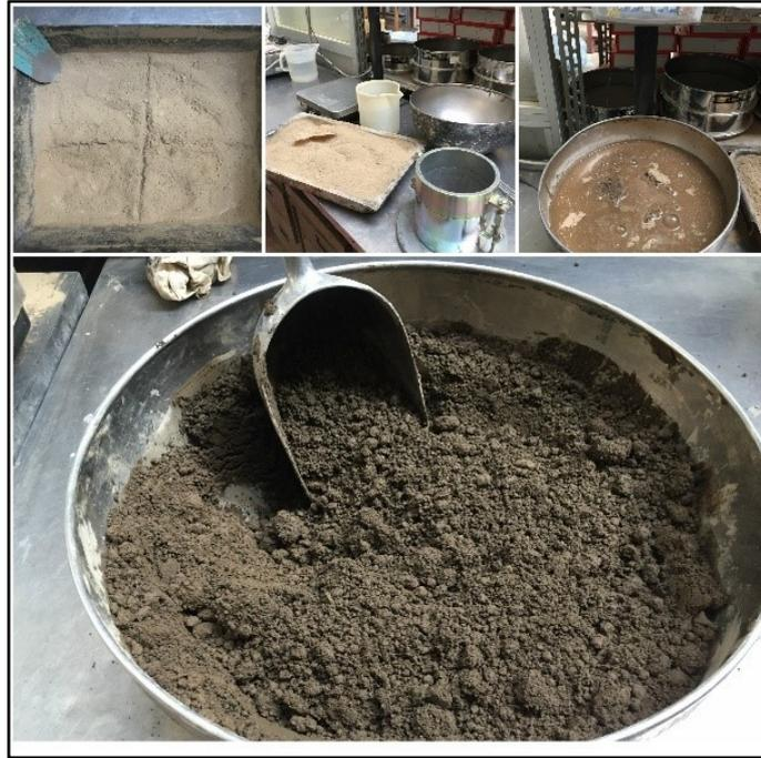
*Fig. 35. Modified Proctor Test*
