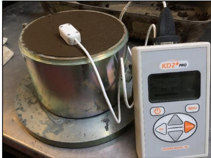
Fig. 39. Thermal Conductivity Measurement of soil A7-6
