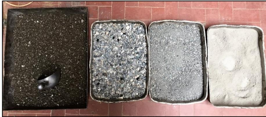
*Fig. 17 Aggregate Used in Aggregate Sludge CLSM*
