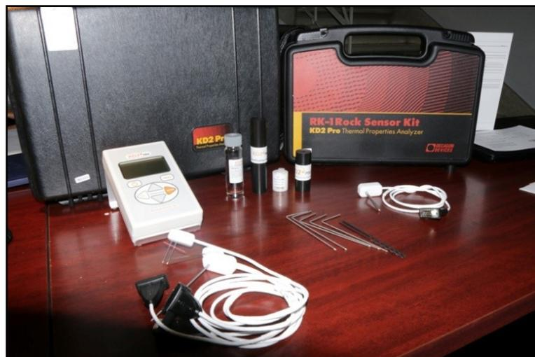
*Fig. 31 KD2 Pro Device with Different Probes and Calibration Cylinders*
