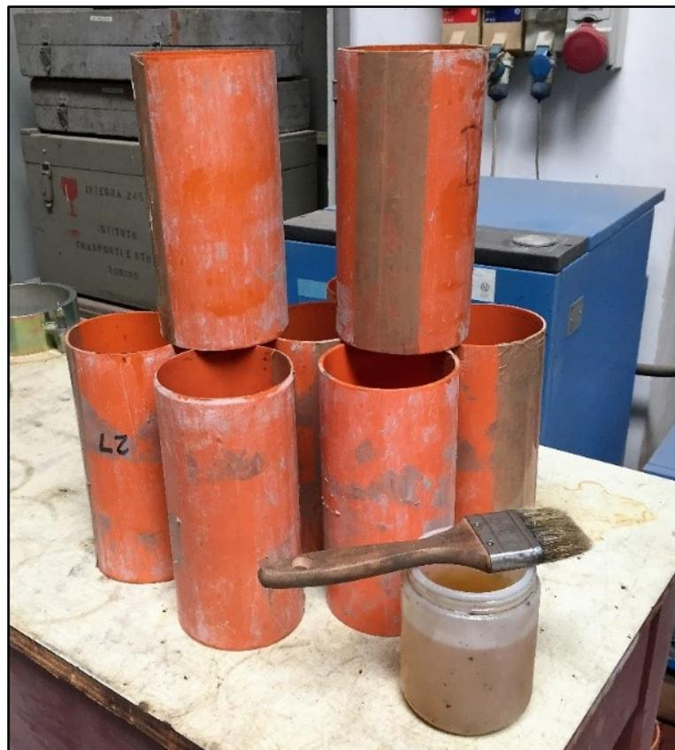
*Fig. 41 Moulds for Casting CLSM*
