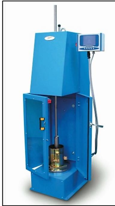
Fig. 28 Automatic Compaction machine[33]
