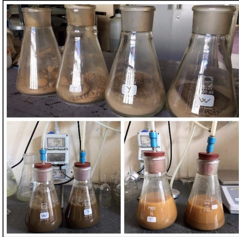
Fig. 34 Pycnometer full of A1-a and A7-6 soil.
