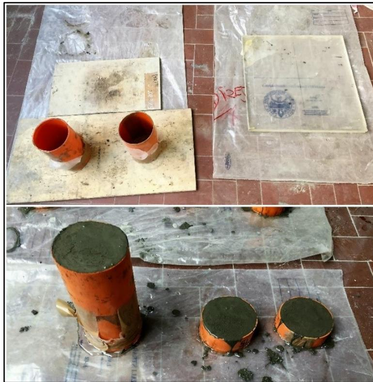
*Fig. 42 Cast CLSM Samples in the Molds*
