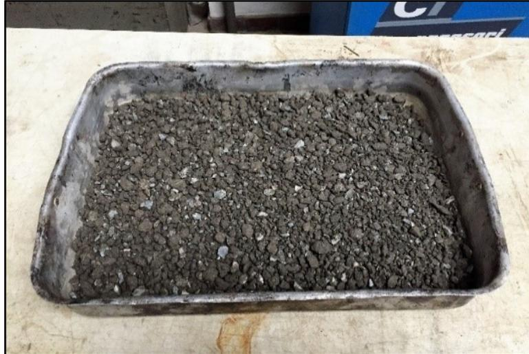
*Fig. 19. RAP material used in laboratory tests*
