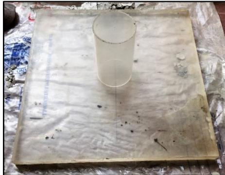
*Fig. 30 Cylinder and plate used for the slump flow test.*
