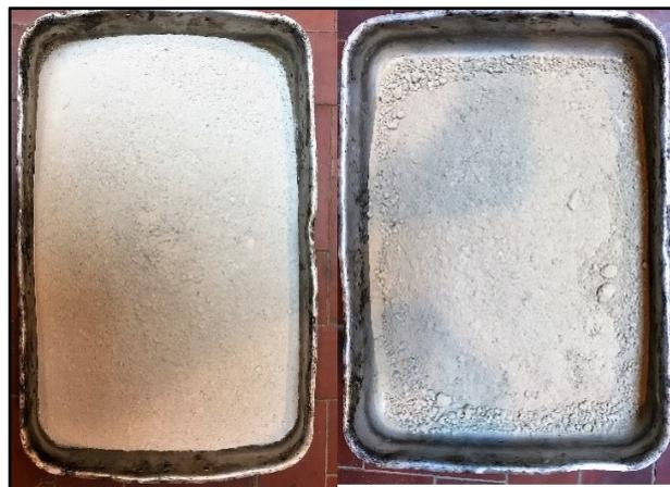
*Fig. 18 Stone Sawmilling Sludge CLSM “A on the right and B on the left”*
