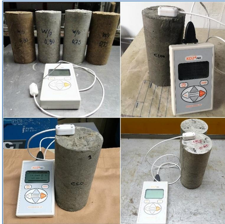
*Fig. 44 Thermal Conductivity Measurement on CLSM's Specimens*
