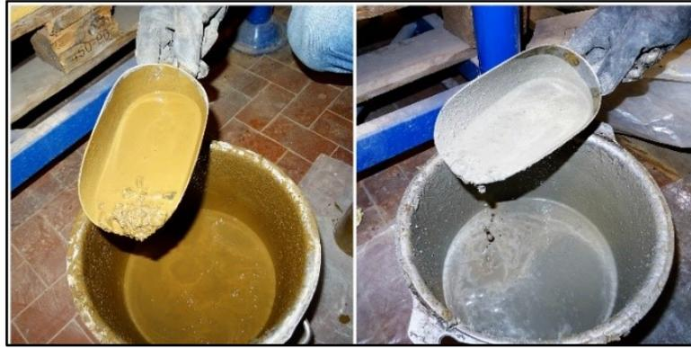
*Fig. 43 Segregation phenomena in Stone Saw Milling Sludge Mixes*
