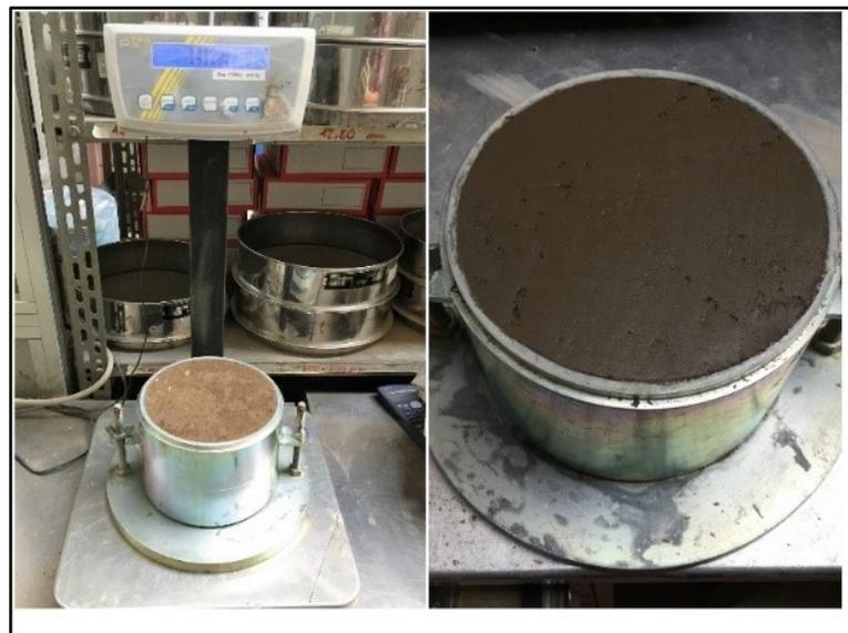
Fig. 37 Flush and Weighing – Modified Proctor Test
