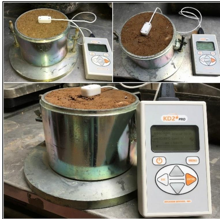
*Fig. 38 Thermal Conductivity Measurement of Soil A1-a*
