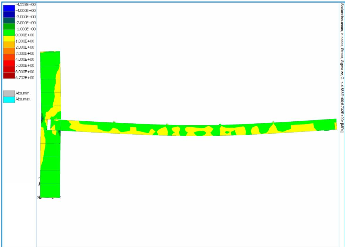
Figure D - 5 Vertical stress  $\sigma_{zz}$  iso-areas Load Case C4
