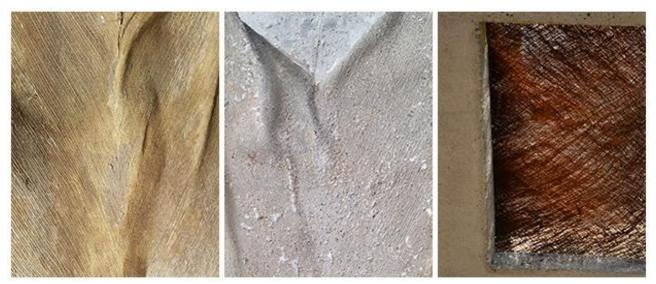
Figure 3: Concrete test with the application of palm fiber to create lights and shadows effects (Natural Sign)
