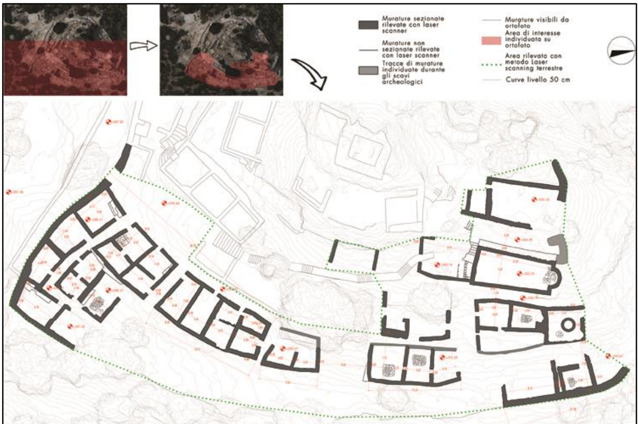
Residential district map, based from the TLS model and superimposed to the 50 cm equidistance contours lines generated from UAV Digital Surface model (DSM). Original scale 1:200
