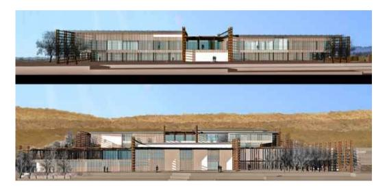
To respect and to honour the Japanese constructive tradition, the wood has been select as project's dominant material for this project. The structure is realized in timber frame, and the fronts are screened by panels of wooden sunshades screening the direct sun.
