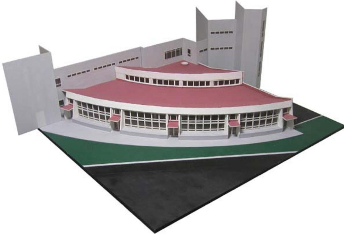
The artificial sky allows to make quantitative assessments: the data acquired by luxmetric probes are elaborated in order to represent illuminance levels through isovalue curves in plan or section and annual trends.
