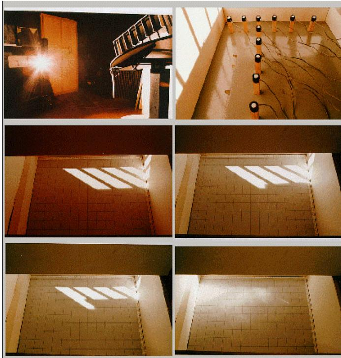
The experimental apparatus and the projected shadows
