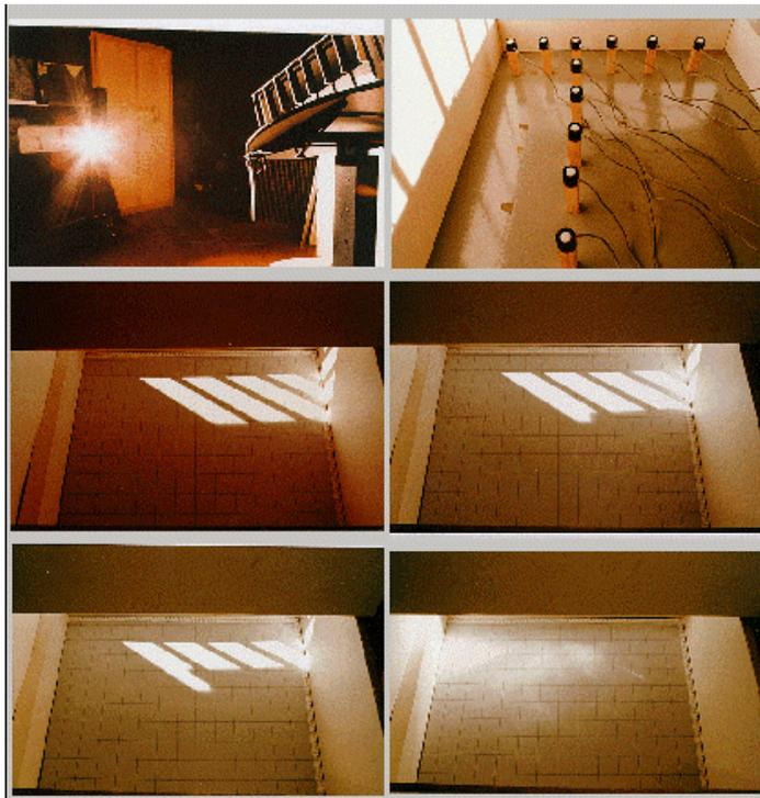
The experimental apparatus and the projected shadows
