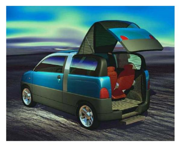
So the interiors are modular, seats are removable and the floor is level, under the floor there is a long space (about 3,80m x 0,60m) that allows you to carry a lot of objects.
