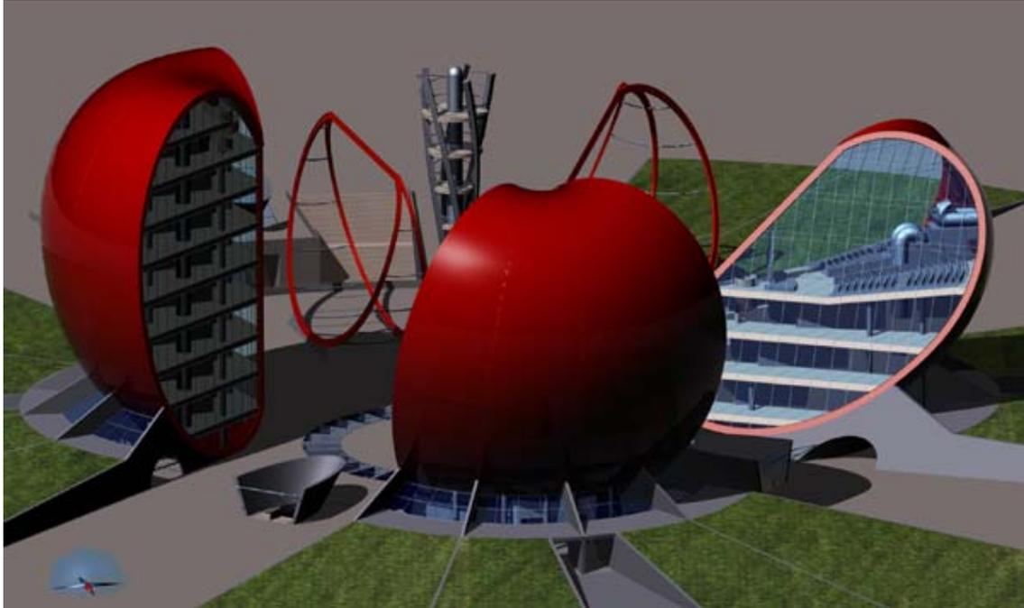
The third building, rotated of 45 degrees, accommodates inside an auditorium served from one winding staircase, one emergency staircase, and an elevator. The beams take the shape of the large ceiling that it traces the shapes of a field of an elliptical arena. The three floors under, with central elevators, have the same outline of the bodies previously described.
