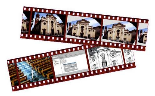
Some phases of the building survey, were done with "Fotogramma" (a software of photographic correction applied in the operations regarding the front of the building), and wiith interfaced total station with the computer during the phases of survey inside the church.
