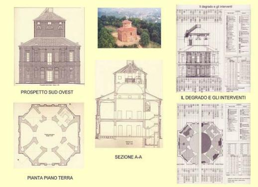
Ground floor plan, significant front view, cross section A-A, example of degradation mapping and intervention.
