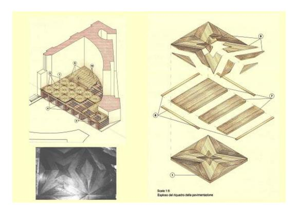
Exploded axonometric view of a significant wooden flooring
