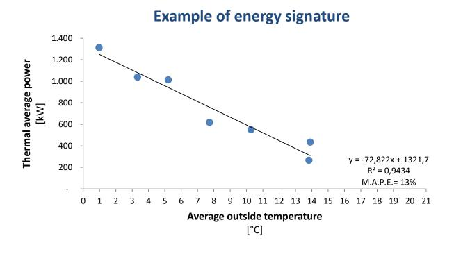
The Figure 1 shows an example of energy signature and in particular the strong linear relationship between consumption and temperature also for analysis at monthly scale. Specifically, the line slope reflects the sensitivity of the building to changes in external temperature and can be compared with building heat transfer coefficient H<sub>tot</sub> [W/K].
