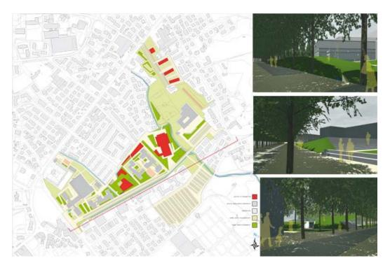
This newly shaped pattern includes the two buildings foreseen by the call for proposals: the auditorium and the library. The library building is located in a barycentric position, and it has been conceived as an extrusion from the surface that creates an overhead square one floor above; all required spaces have been carefully "cut" into it.
