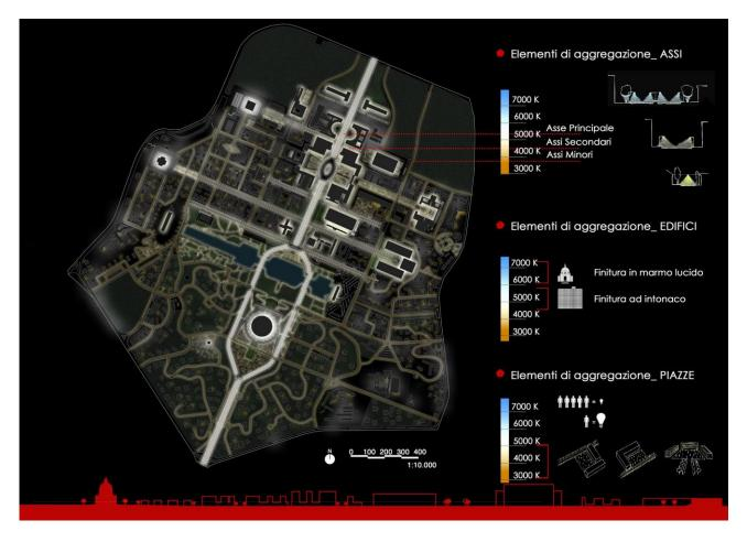
**Figure 2 –** Urban lighting masterplan of the Eur district. It highlights the differentiation in the use of the color temperature of the light, in order to create hierarchies among the elements constituting the urban plot.
