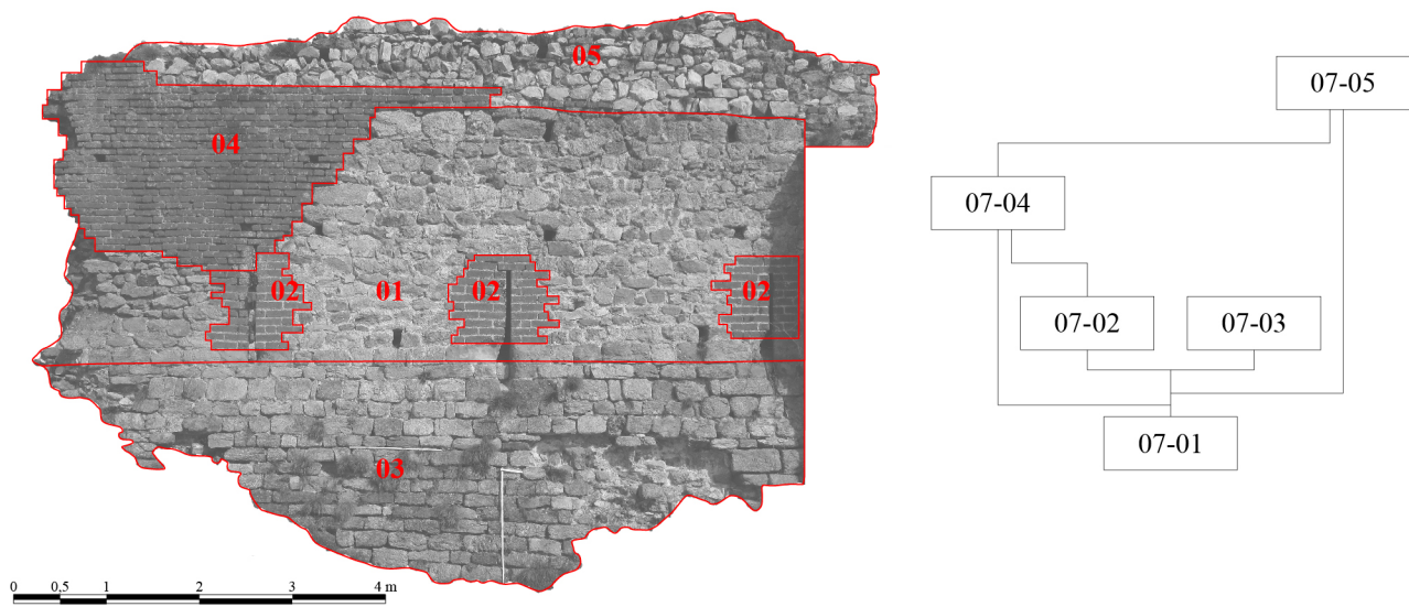
Fig.3 – Example of subdivision of one wall of the castle and, on the right side, the matrix
