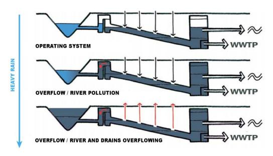
Schematics of the spill in a sewage system
