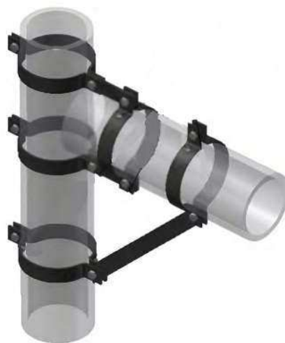
Immagine 39. Connessioni tramite fascette metalliche, Data source: Bamboo joints with steel clamps capable of transmitting
