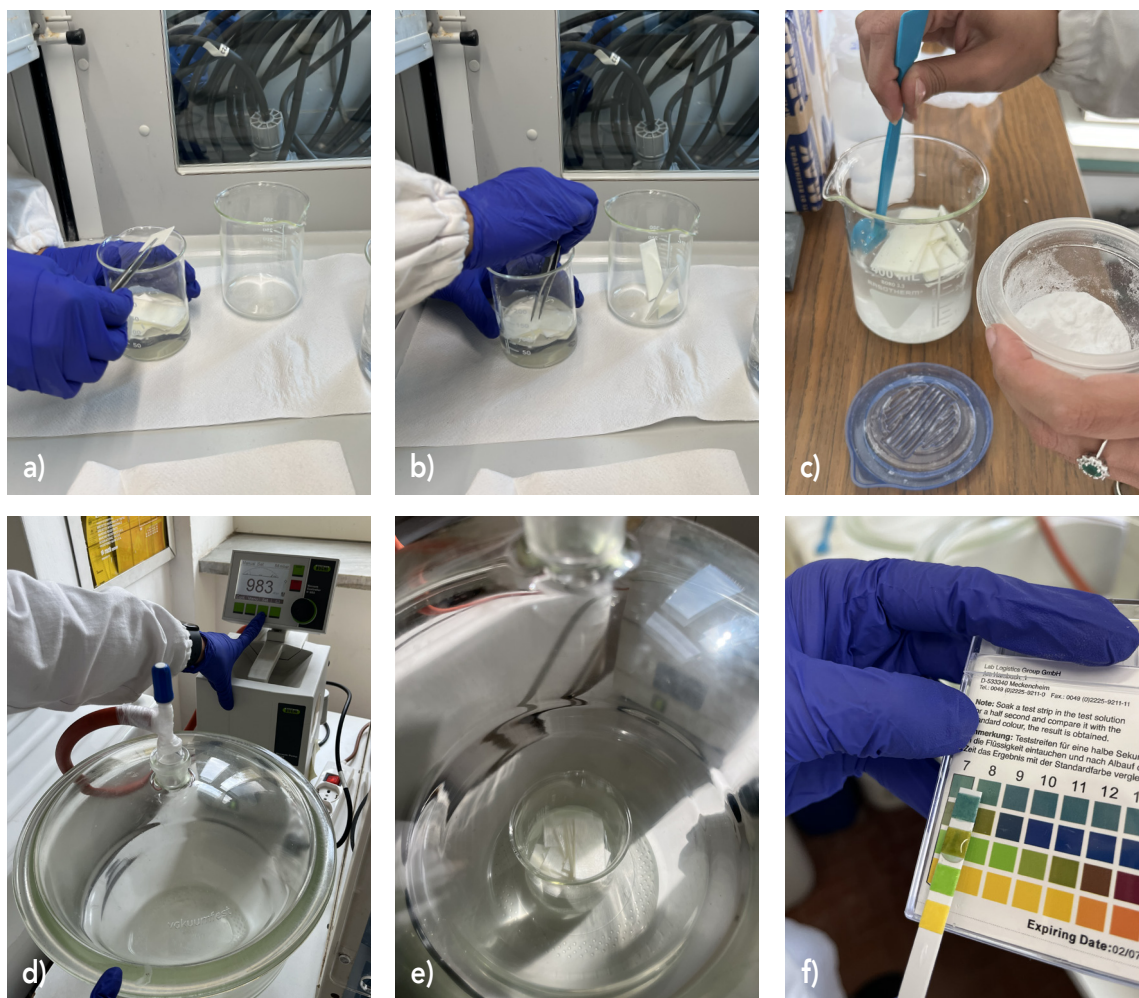
Figure 18. (a) (b) Transferring the samples into a new beaker; (c) Washing solution; (d) Vacuum chamber; (e) Washing cycle under vacuum conditions; (f) pH test strip comparison. Photos taken by the author in the laboratory at Politecnico di Torino.
