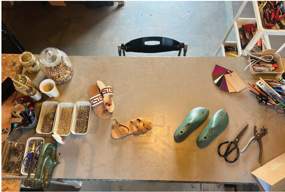
Fig. 73 Contemporary sandal prototyping workspace showing material experimentation and fabrication processes. On the central worktable are early mock-ups inspired by ancient Greek footwear, assembled alongside lasts, leather samples, hardware components, fasteners, and cutting tools. The arrangement highlights the translation of archaeological references into present-day craft practice, where historical typologies are tested through modern construction methods, ergonomics, and material performance.
