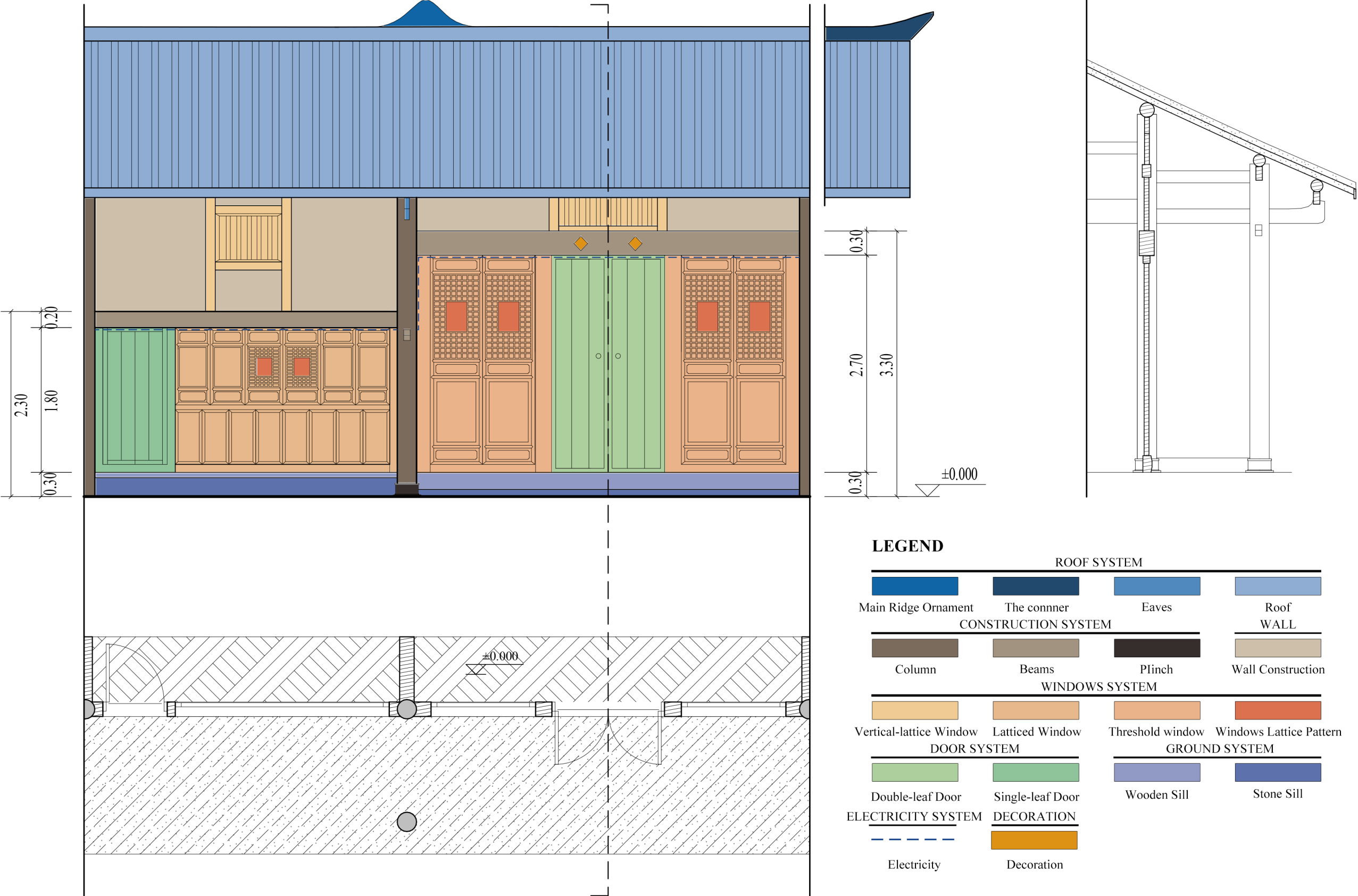
Image 82 Construction Element of Selected Facade Scale 1:50 Draw by Author
