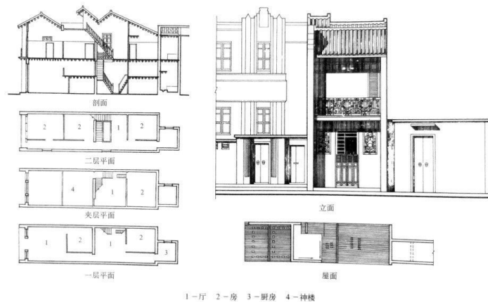
Figure 3-14 Typical Bamboo Tube House Plan, Elevation and Section Source; Lu Yuanding and Wei Yanjun's "Guangdong Folk Houses"
