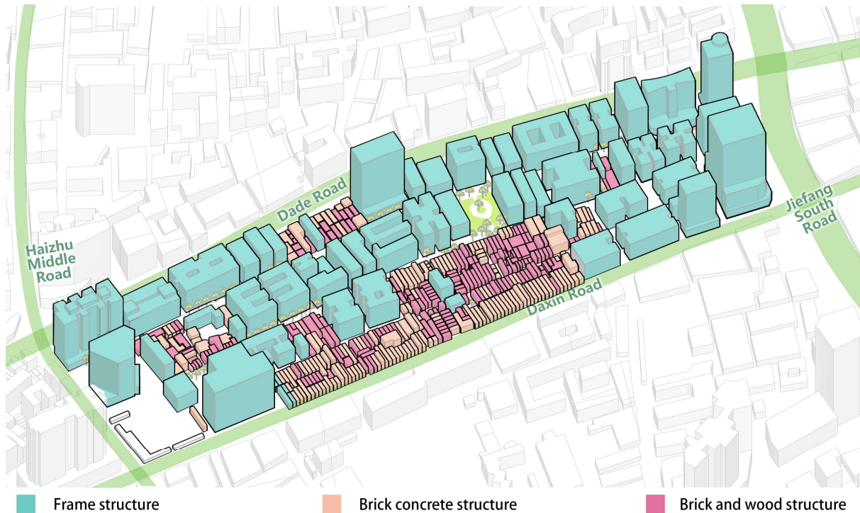
Figure 4-23 Types of Building Structures Around Haopan Street Source: Author's drawing
