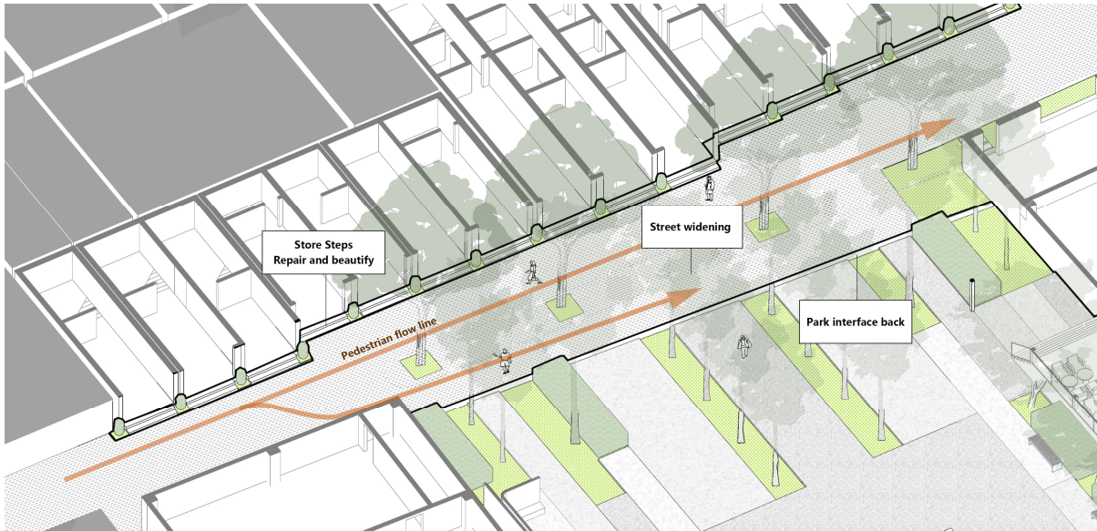
Figure 5-27 Street Node 2 Axonometric Drawing After Renovation Source: Author's drawing
