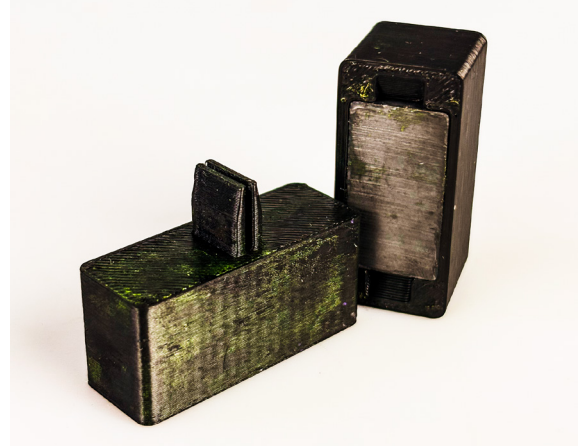
Fig. 117 Sliders and magnetic slider for movable types
