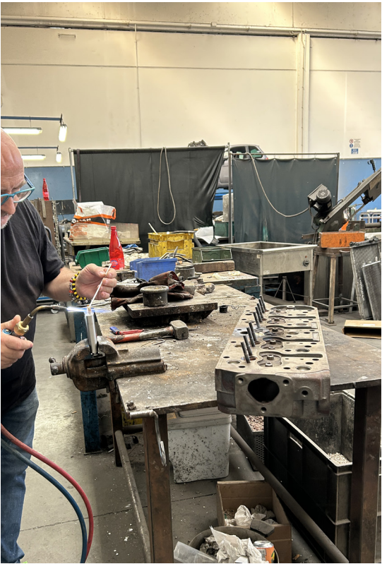
Left page: tests for the new fitting between the flask and the tubes of the water system. Top left: interior view of the first and second modules to determine the fitting placement. Bottom left: copper fitting soldered to the stainless steel flask. Right: soldering of the copper fitting to the stainless steel flask carried out by Nuova Salderia S.r.l.
