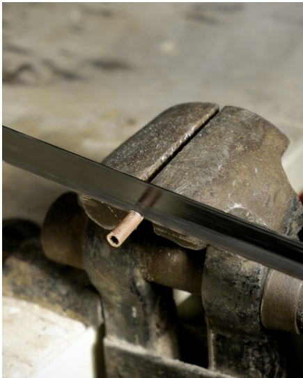
Left page: soldering the copper tubes using the kitchen gas stove. Top left: internal copper components of the second module. Bottom left: cutting the copper tubes. Top right: workbench with the second module and the new copper tubes and fittings.
