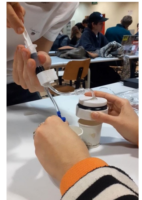
Left: lifting 9 kg with a syringe to reach 9 bar of pressure. Right: water system with one-way valves.
