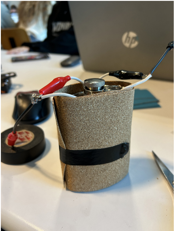
Top: the first welds of the battery system. Bottom left: temperature measurement to test the insulating materials. Bottom right: the external insulation made of cork.
