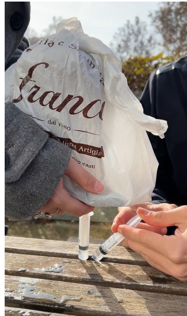
Left: lifting 9 kg with a syringe to reach 9 bar of pressure. Right: water system with one-way valves.
