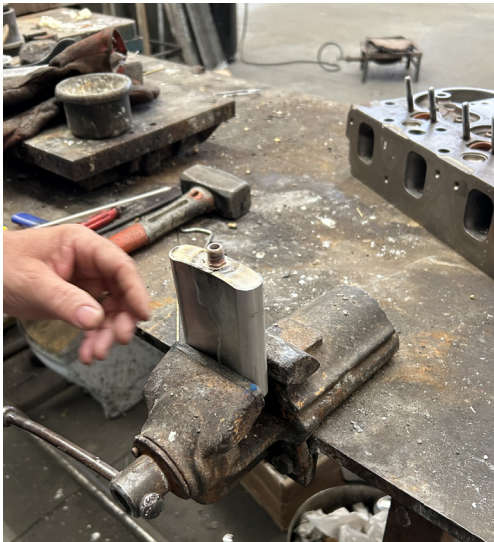
Left page: tests for the new fitting between the flask and the tubes of the water system. Top left: interior view of the first and second modules to determine the fitting placement. Bottom left: copper fitting soldered to the stainless steel flask. Right: soldering of the copper fitting to the stainless steel flask carried out by Nuova Salderia S.r.l.
