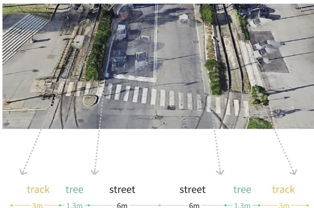
Figure 59a. Widths of different components of east road section used for modeling
