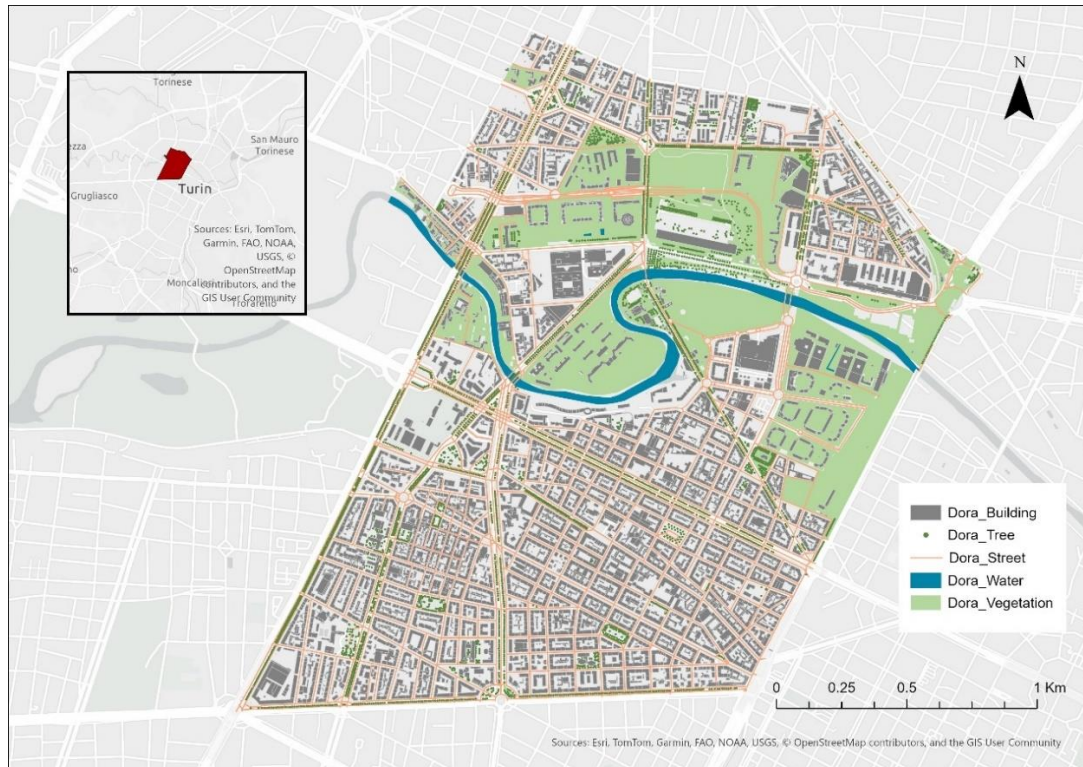
Figure 41. The resulting vector data obtained through Clip tool contain only the spatial features located within the study area.
