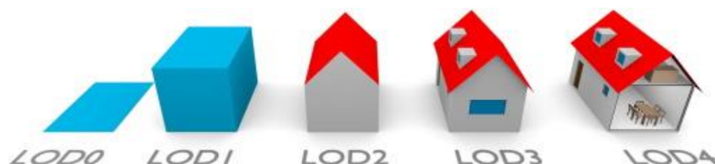
Figure 43. The five LODs gradually increase in geometric detail and semantic complexity, with LOD4 ultimately containing indoor features.
