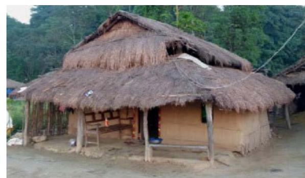
Figura 82. "Tharu house with wide roof overhang and shaded veranda".
