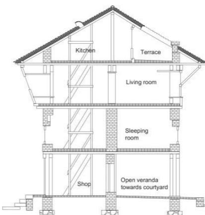
Figura 85. "Section of Newar house with vertical space arrangement".
