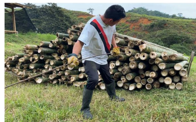
Figura 63. "Puncturing holes in all the nodes of the bamboo".
