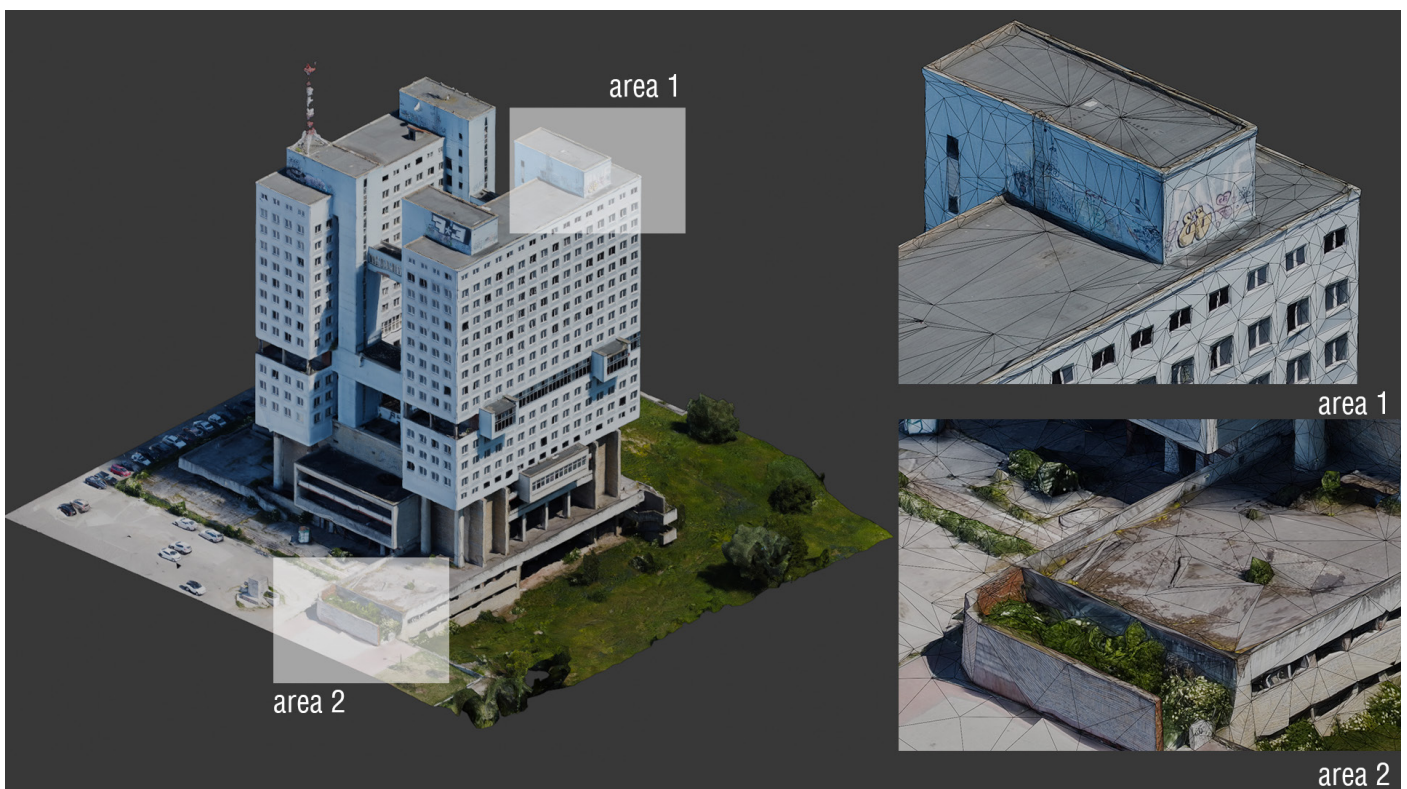
Figure 11. The House of Soviets model with 89,000 polygons after applying Decimate. Area 1 and Area 2—mesh density and texture quality. Source: Ivan Karnitckii 2025.
