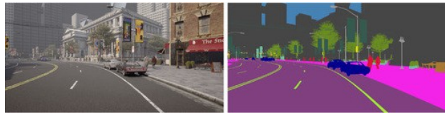
Figure 2.4: Example of semantic segmentation , where each pixel is assigned to a class (e.g. road, car, sky).
