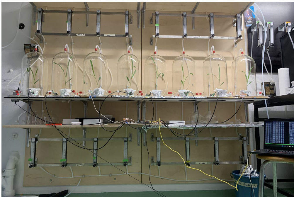
Figure 3.12: Laboratory configuration for maize herbivory VOC sampling.
