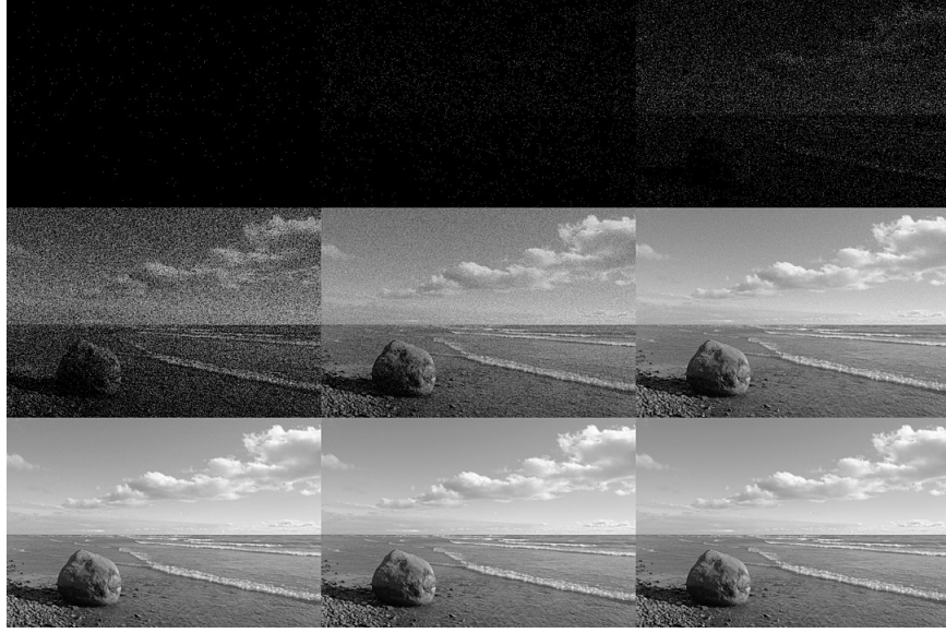
Figure 2.1: Effect of shot noise. Number of photons per pixel increases from left to right and from top to bottom. Image from: https://en.wikipedia.org/wiki/Shot_noise
