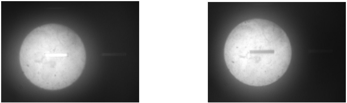
Figure 5.8: Since the BSW is TE polarized, we can see the gratings switching on and off, depending on the incident light's polarization. On the left TE, on the right TM.
