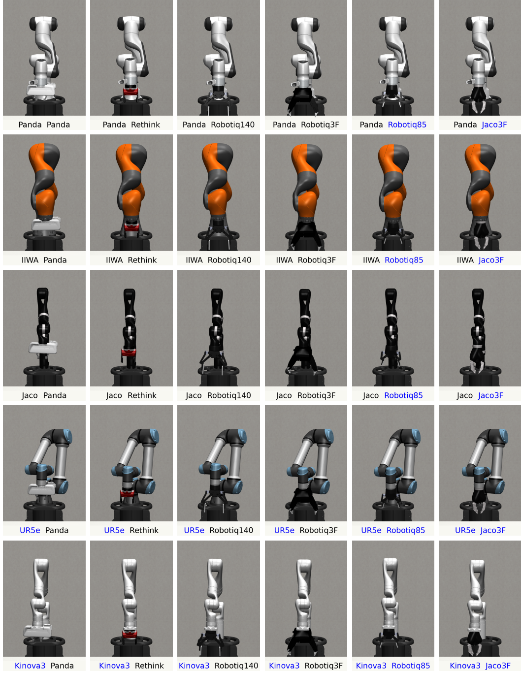
Figure A.4: Visualization of all robot-gripper configurations ( 5 \text{ robots} \times 6 \text{ grippers} ) considered in the experiments with the vision-based policy. The unseen components during training are reported in blue in the titles of each image.
