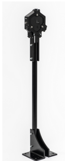
Figure 6.4: Front view of the load cell assembly: left image shows Flight Stand 15 load cell, right image shows detailed component in front view, ref [37].
