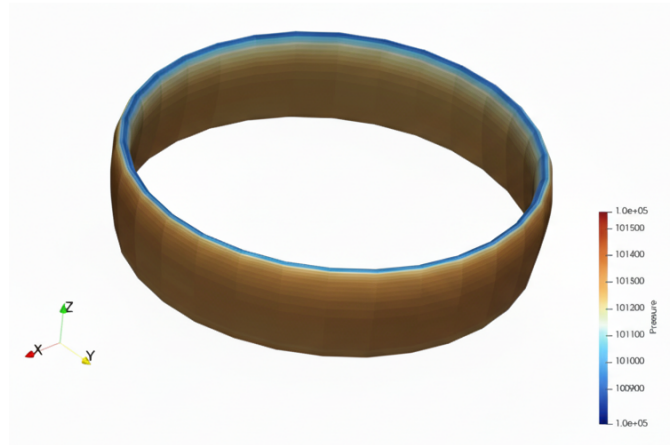
Figure 5.12: Pressure distribution along the duct from ParaView
